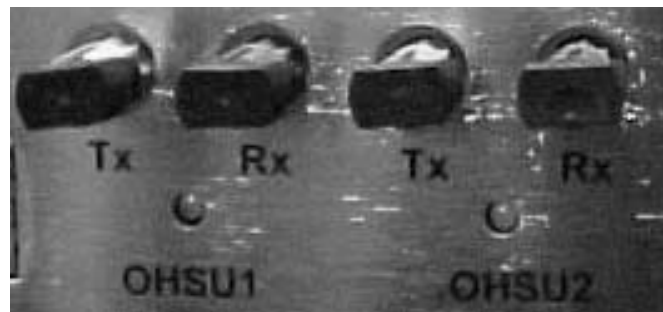
Figure 10-1. Optional two-Port OHSU port
