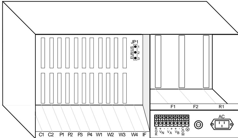
Figure Slot-4. Front-Loading Chassis - Power Supplies on Side (newer model)
