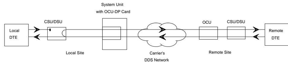
**Figure OCU-8. OCU Remote Loopback (csu-u option)**
