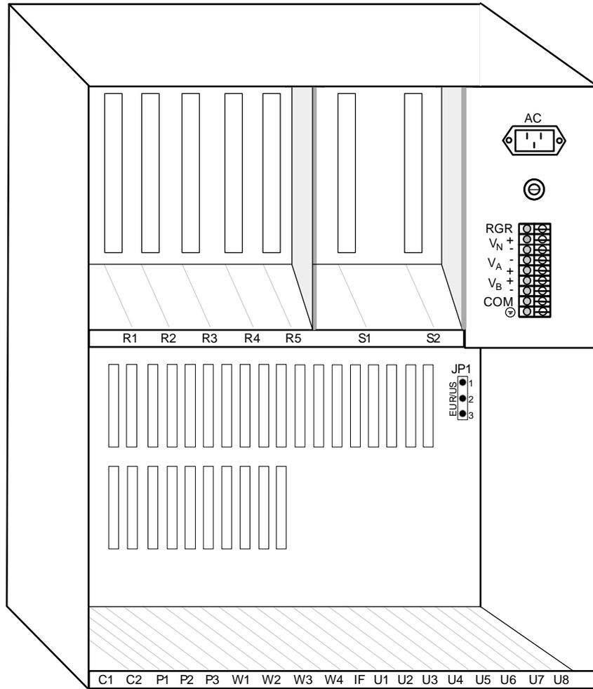
**Figure Slot-5. Front-Loading Chassis - Power Supplies on Top**
