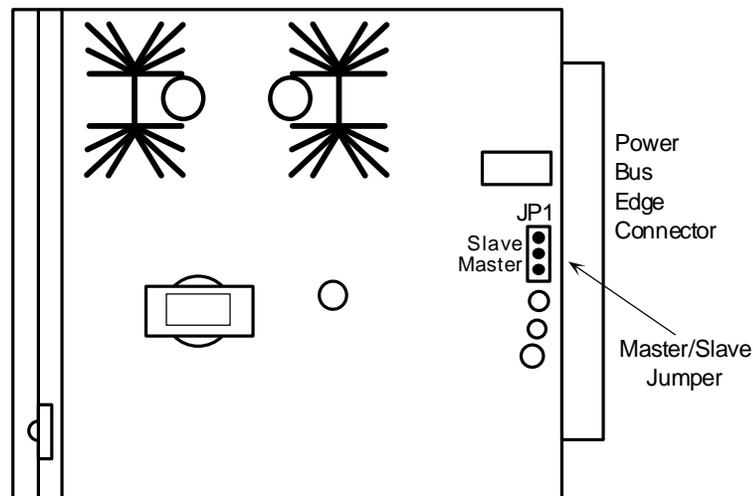
Figure Install-18. 8906 Ringing Generator Layout
