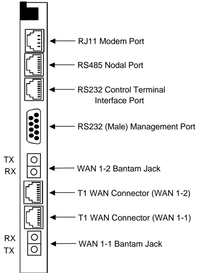
Figure Pinouts-11. 8926 Interface Card Port
