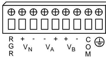
Figure Install-13. 891620 Terminal Power Connector
