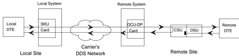
**Figure SRU-5. A Remote CSU Loopback Commanded by the System**
