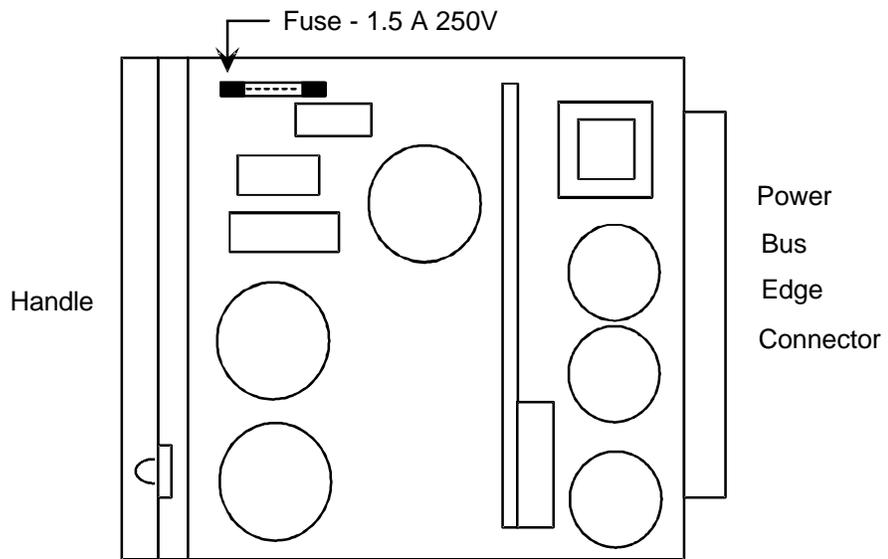
Figure Install-16. AC-to-DC Converter Layout
