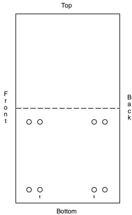
**Figure Install-4. Mounting Holes (Front-Loading Chassis, Power Supplies on Top)**
