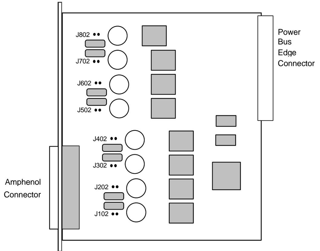
Figure BRI-14. Sealing Current Jumper Locations on the 8261 BRI Card
