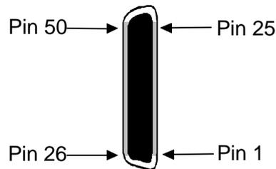
**Figure Pinouts-13. External Alarm Card Connector Pinouts**
