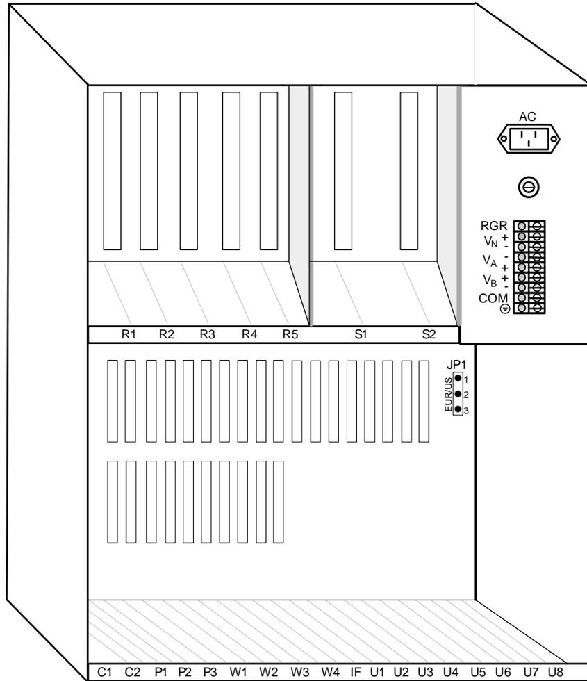
Figure Pinouts-5. 891920 Front-Loading Chassis.
