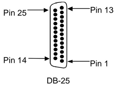
**Figure Pinouts-29. Channels 1 and 2 Connectors on 8202 HSU Card**
