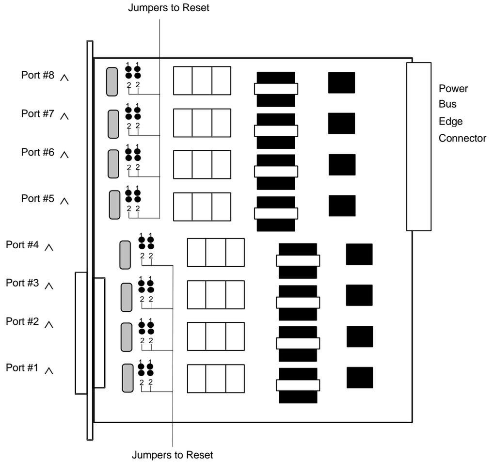
Figure FXO-4. Jumpers for mrd Mode
