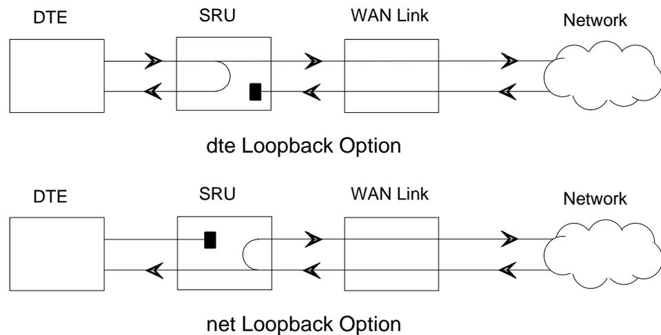
Figure SRU-3. SRU Card Loopbacks
