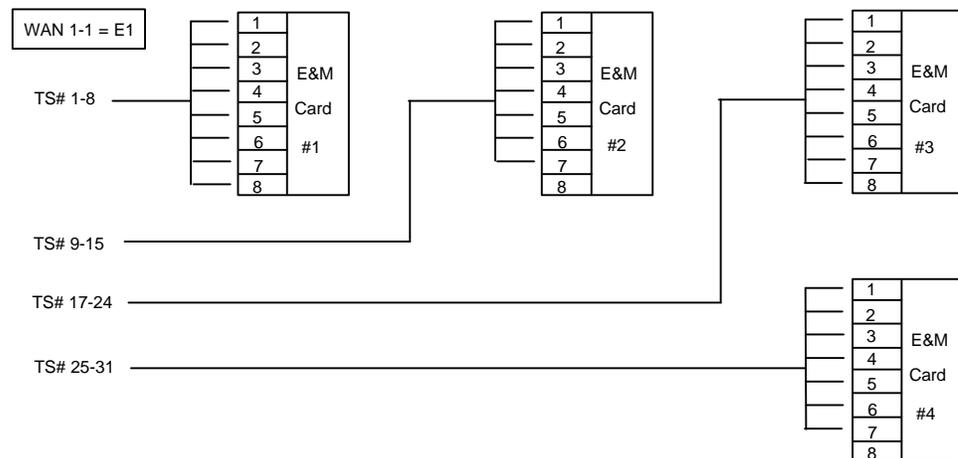
**Figure System-4. Timeslot Map Using Configuration Option in E1 Operation**
