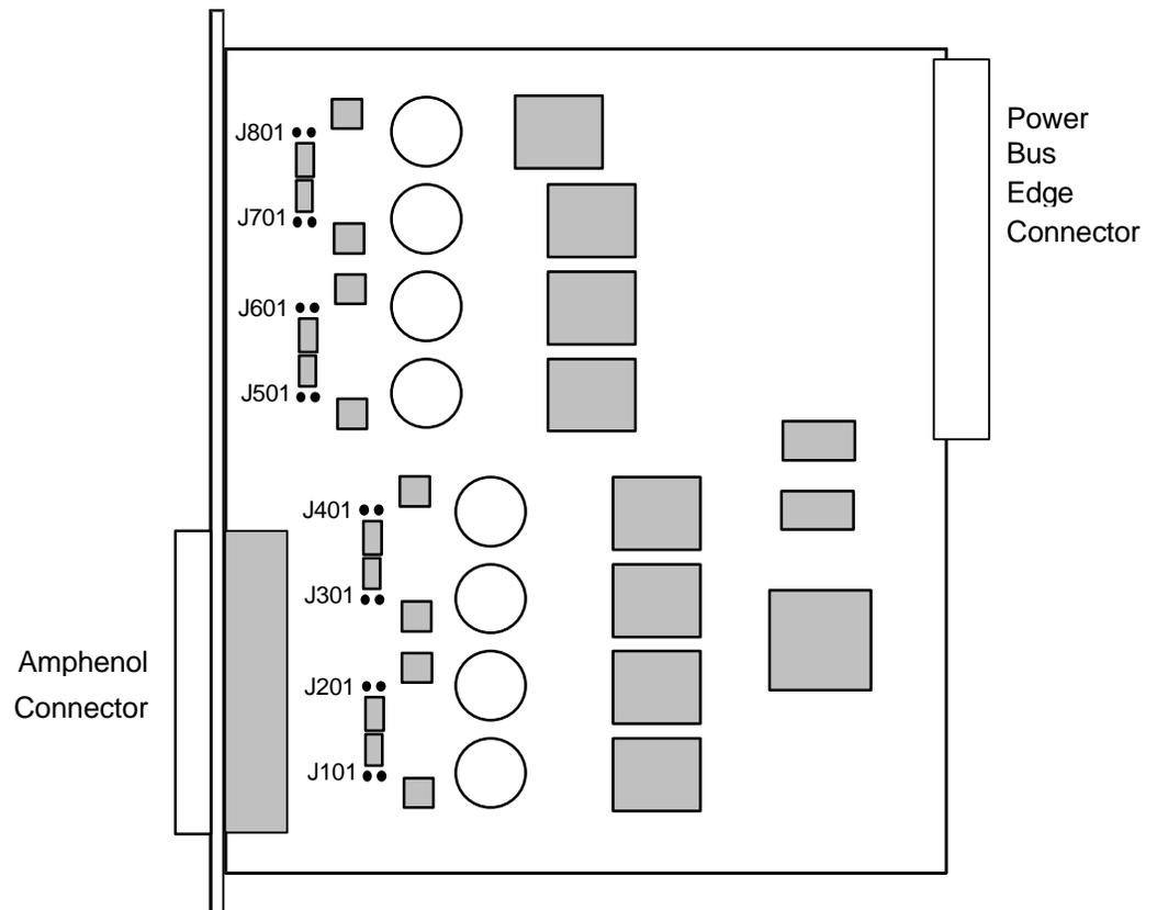
Figure BRI-13. LT-NT Jumper Locations on the 8261 BRI Card
