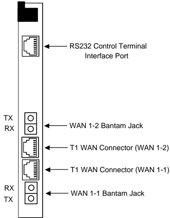
Figure Interface-3. 8925 Interface Card Ports
