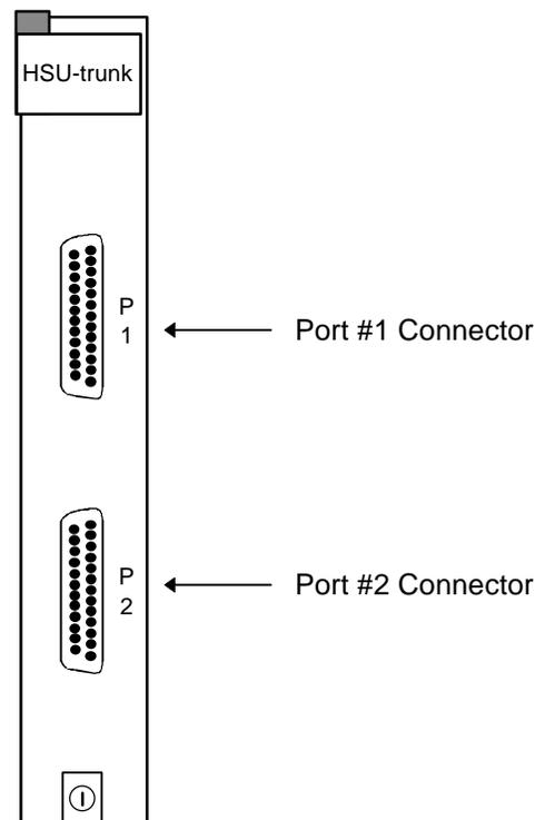
Figure Pinouts-34. 8214 HSU Card Connectors
