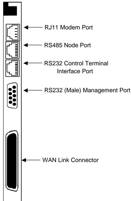
**Figure Pinouts-6. Interface Card Connectors (8920 and 8921)**
