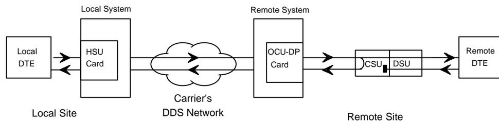
**Figure HSU-8. A Remote CSU Loopback Commanded by the System**
