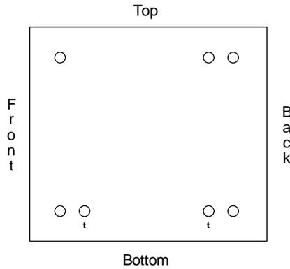
**Figure Install-2. Mounting Holes (8916 Front-Loading Chassis)**
