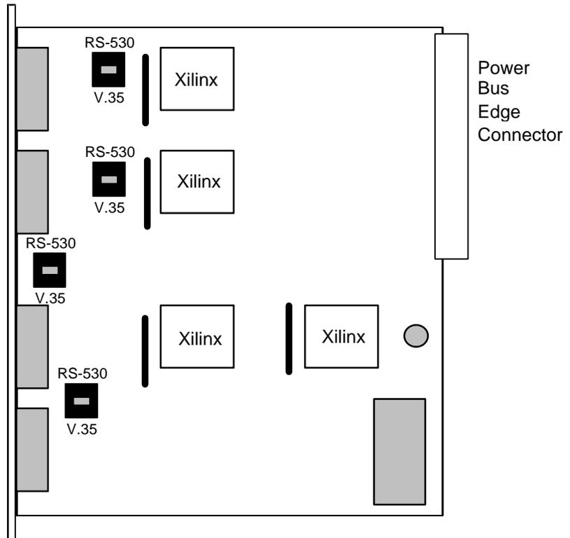
Figure HSU-11. Switches for Conversion from RS530 to V.35
