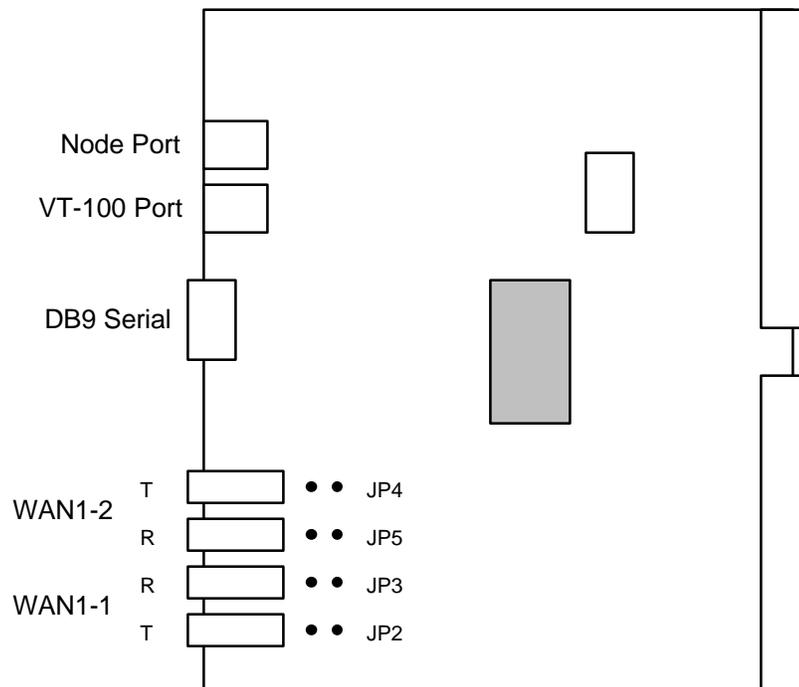
**Figure Interface-11. Jumpers on the 8927 Card**
