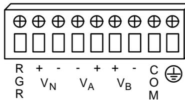
Figure Install-14. 891822/891823 Terminal Power Connector
