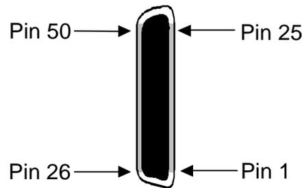
Figure Pinouts-45. BRI Card Connector
