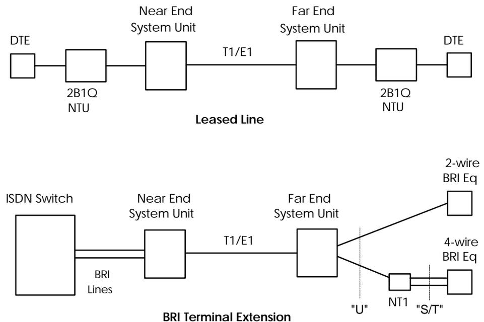
Figure BRI-1. Typical BRI System Application
