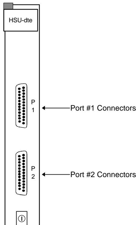
Figure Pinouts-30. 8203 HSU Card Connectors
