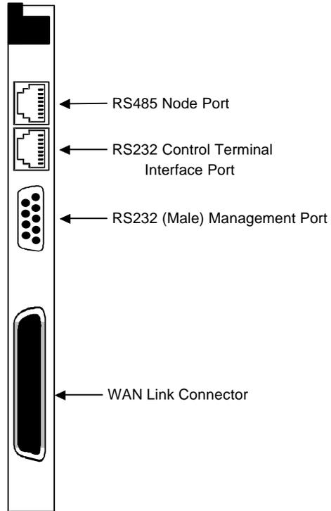
**Figure Interface-2. 8921 Interface Card Front Panels**
