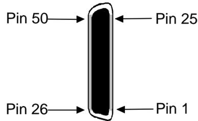
**Figure Pinouts-25. 8138 and 8139 FXO Card Connector**
