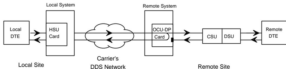
**Figure HSU-7. A Remote OCU or DS0 Loopback Commanded by the System**
