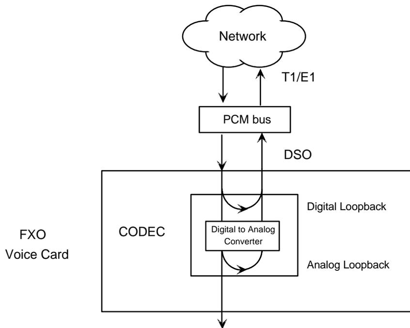
Figure FXO-2. FXO Card Loopbacks
