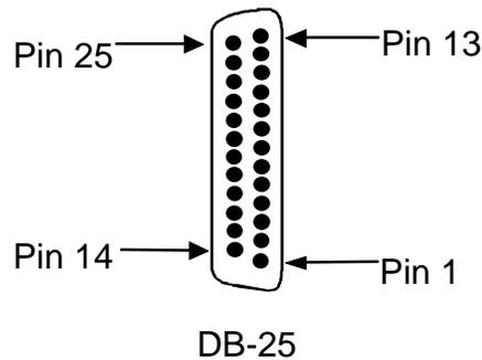
**Figure Pinouts-35. Connectors on an 8214 HSU Card**
