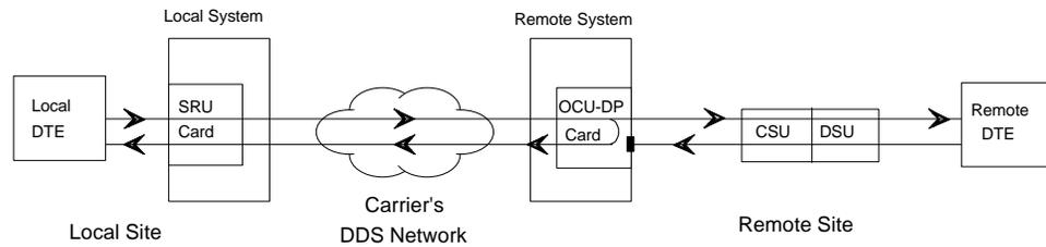
**Figure SRU-4. A Remote SRU Loopback Commanded by the System**
