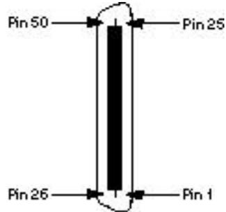
Figure Pinouts-26. FXS Coin Card Jack
