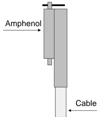
**Figure Install-19. Undesirable Amphenol Connectors**
