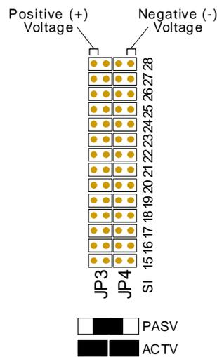
**Figure Pinouts-16. Jumper Pair Assignments.**
