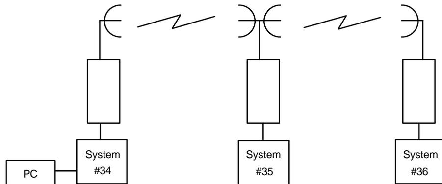
**Figure Interface-10. Typical RTS Configuration**
