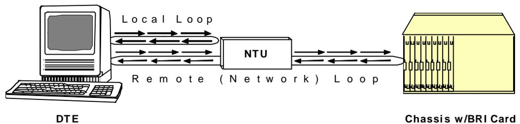
Figure BRI-6. Local and Remote NTU Loopback Testing.
