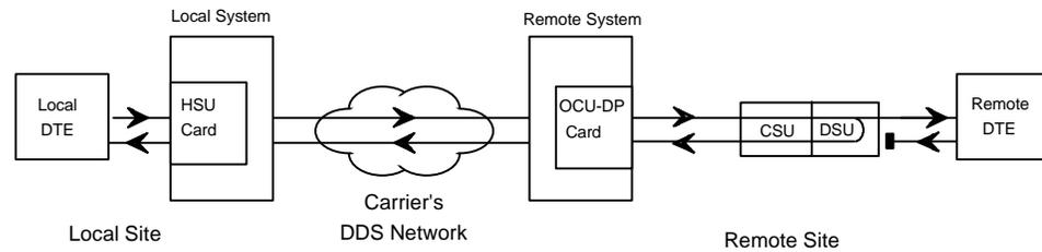
**Figure HSU-9. A Remote DSU Loopback Commanded by the System**
