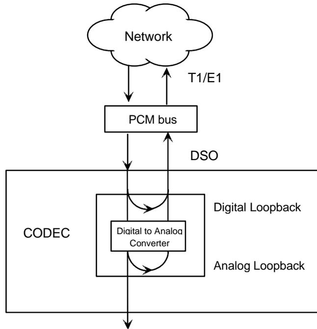
Figure FXSC-2. FXS Coin Card Loopbacks
