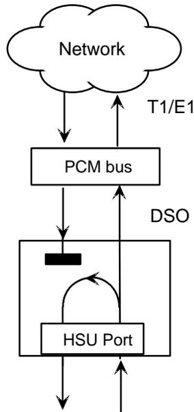
**Figure HSU-5. Data Card DTE Loopback**
