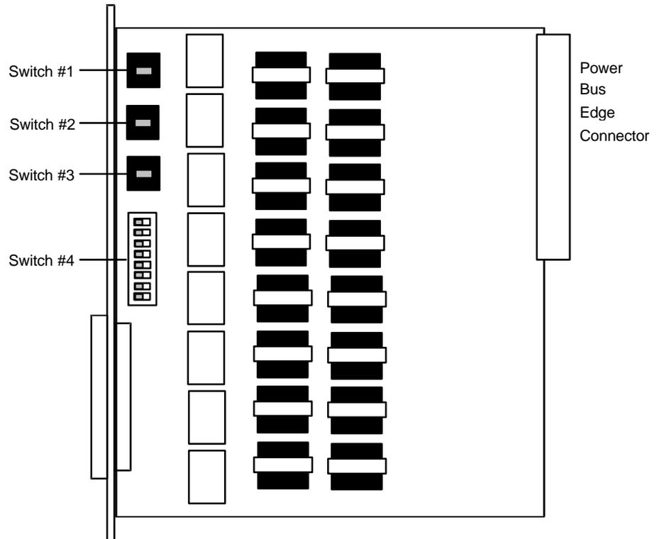
**Figure E&M-1. Positions of the four E&M Card Switches**
