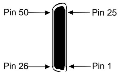
Figure Pinouts-15. External Alarm Card (8403) J3/J4 Pinouts
