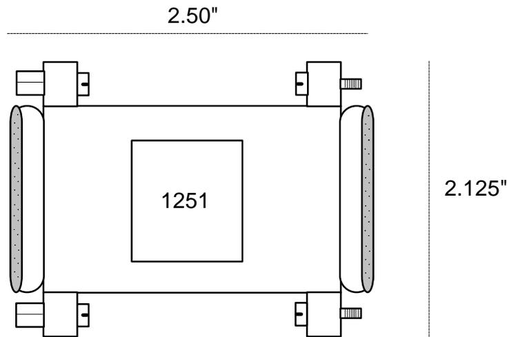
**Figure HSU-12. The RS530 to V.35 Personality Module**
