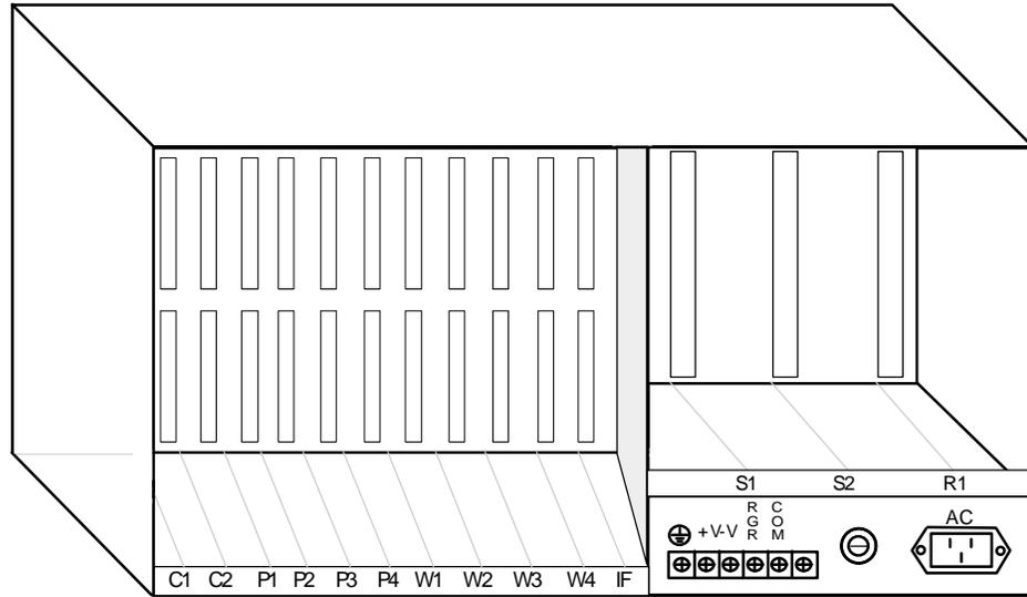
Figure Slot-3. Front-Loading Chassis - Power Supplies on Side (older model)
