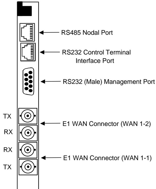
Figure Pinouts-12. 8927 Interface Card Port
