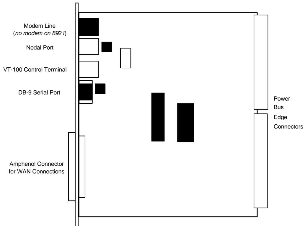
**Figure Interface-6. Component Layout for the 8920 and 8921 Interface Card**
