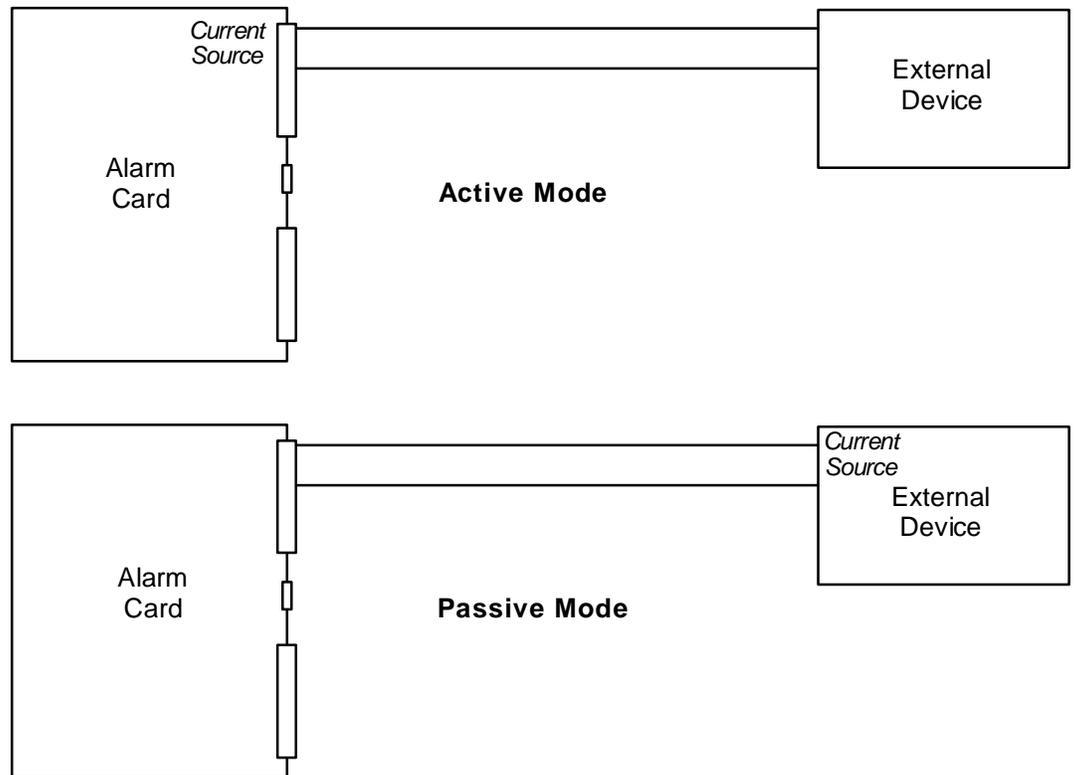
Figure Alarm-6. Active Mode vs. Passive Mode.
