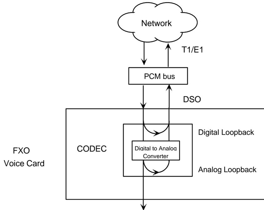
**Figure FXOC-3. FXO Coin Card Loopbacks**
