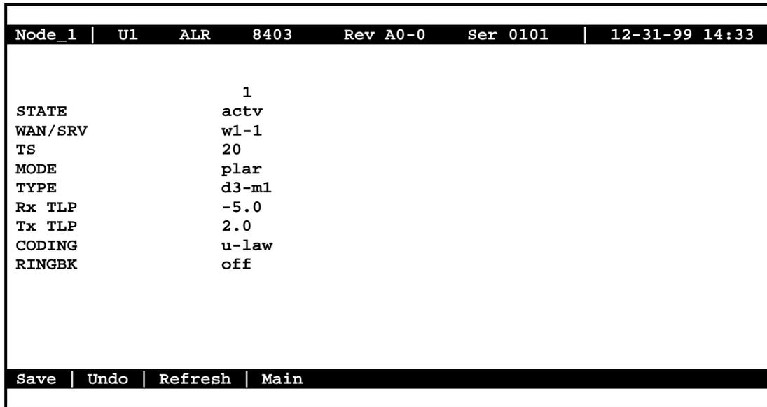
Figure Alarm-4. External Alarm Card (8403) Voice Screen
