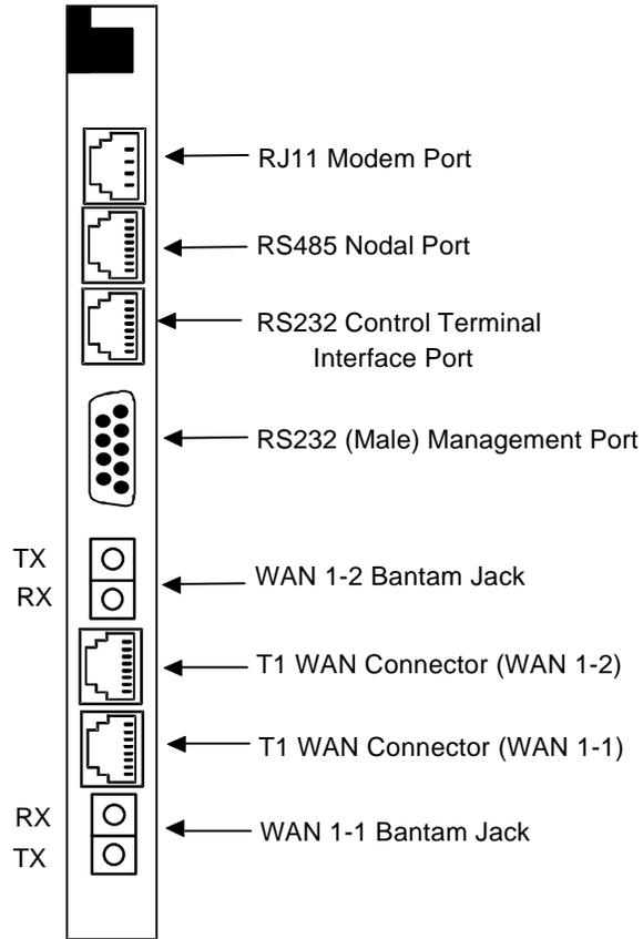
Figure Interface-4. 8926 Interface Card Port
