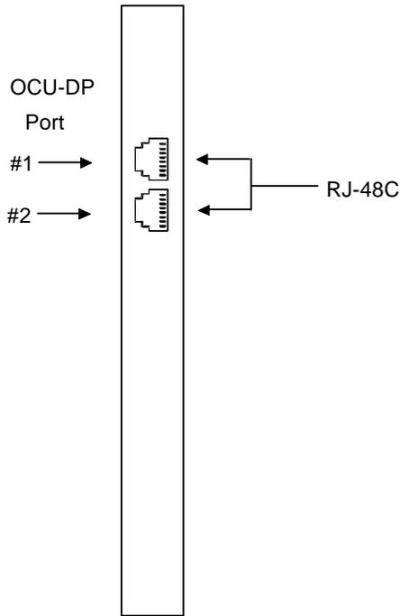
**Figure Pinouts-41. 8249 OCU-DP Card Connectors**
