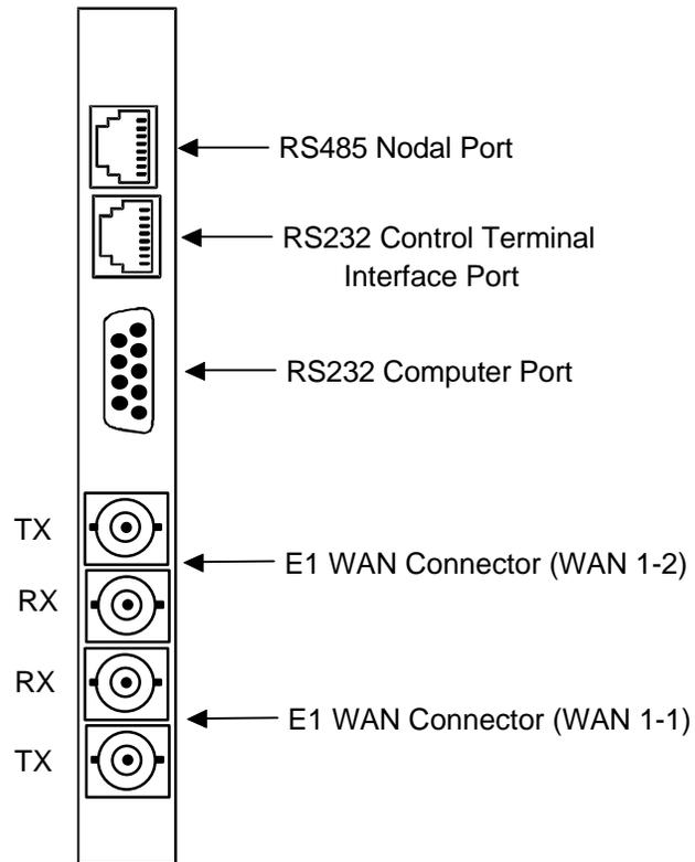
**Figure Interface-5. 8927 Interface Card Port**
