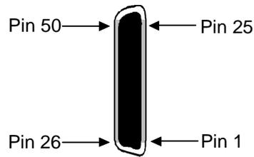
Figure Pinouts-7. WAN Link Connector
