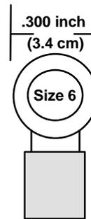
**Figure Install-12. Ring Terminal (insulated) Specifications**
