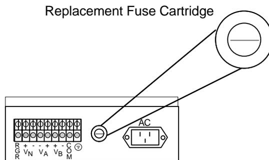
**Figure Slot-6. Replacement Fuse Cartridge on Chassis**
