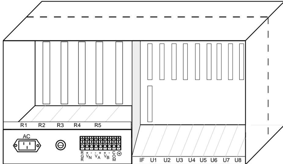
Figure Slot-2. Two-Sided Chassis - Rear View
