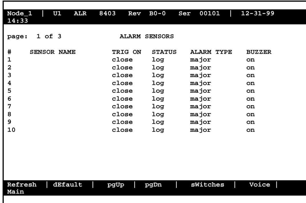
Figure Alarm-2. External Alarm Card (8403) Sensors Screen
