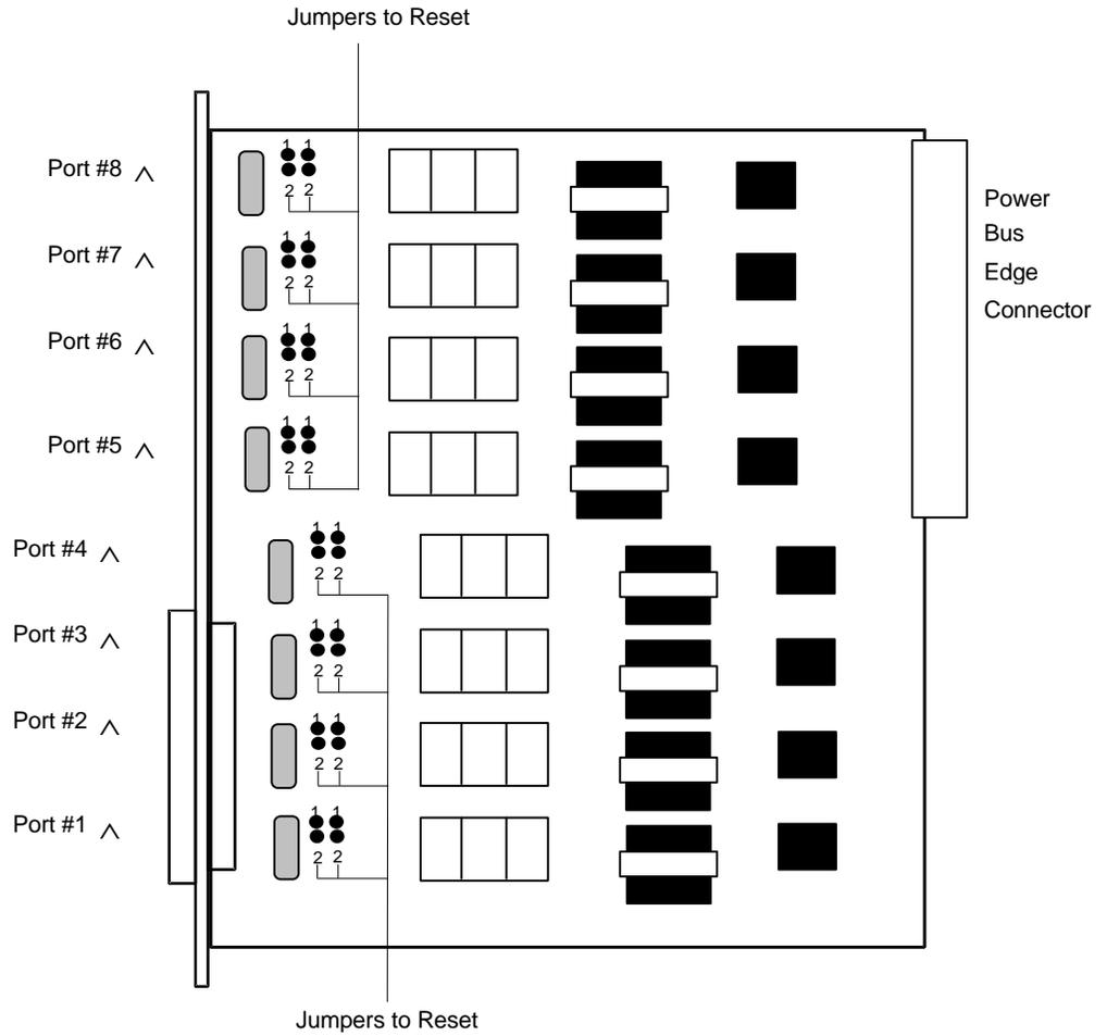
Figure FXOC-1. Jumpers for mrd Mode
