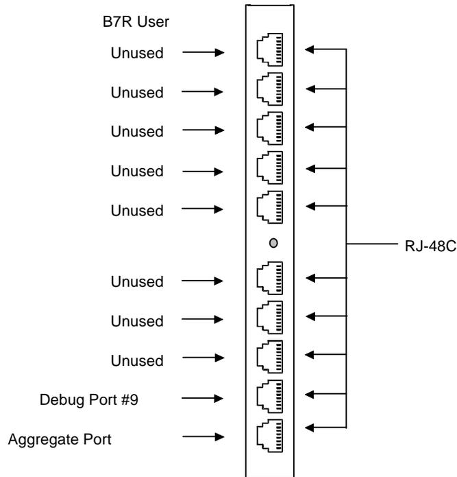
**Figure Pinouts-44. B7R Card Connectors**
