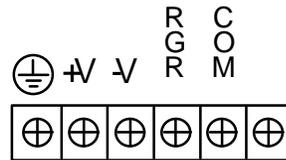
**Figure Install-11. 8916 External Power Connector (rev. C1+)**
