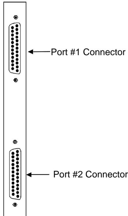
Figure Pinouts-32. 8212 HSU Card Connectors
