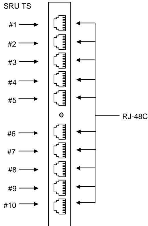
Figure Pinouts-38. SRU Card Connectors
