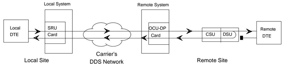
**Figure SRU-6. A Remote DSU Loopback Commanded by the System**
