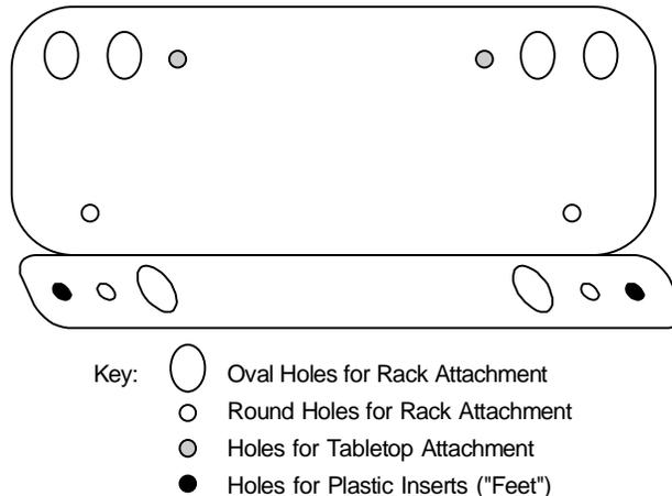
**Figure Install-5. Hole Pattern on the Mounting Bracket**
