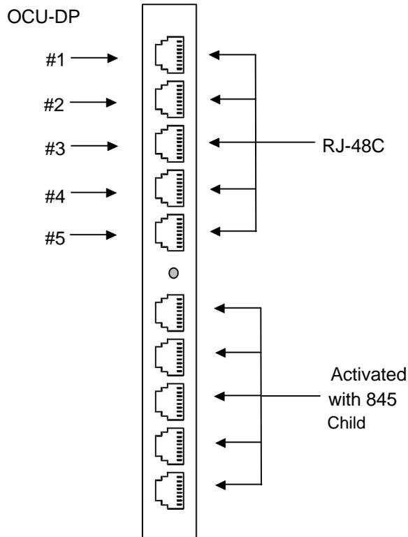
Figure Pinouts-40. 8248 OCU-DP Card Connectors
