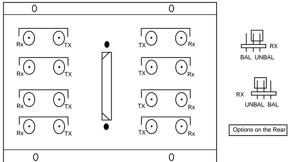
Figure Pinouts-9. 1184 E1 Interface Adapter
