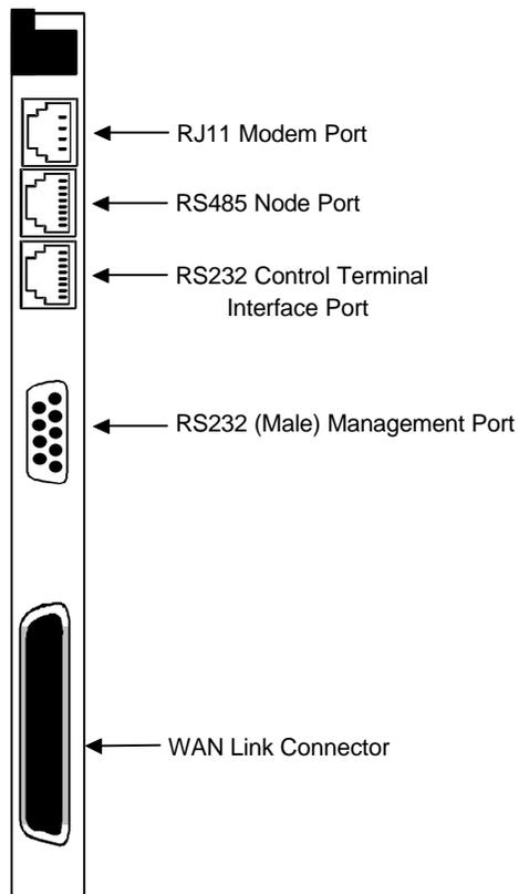
**Figure Interface-1. 8920 Interface Card Front Panels**
