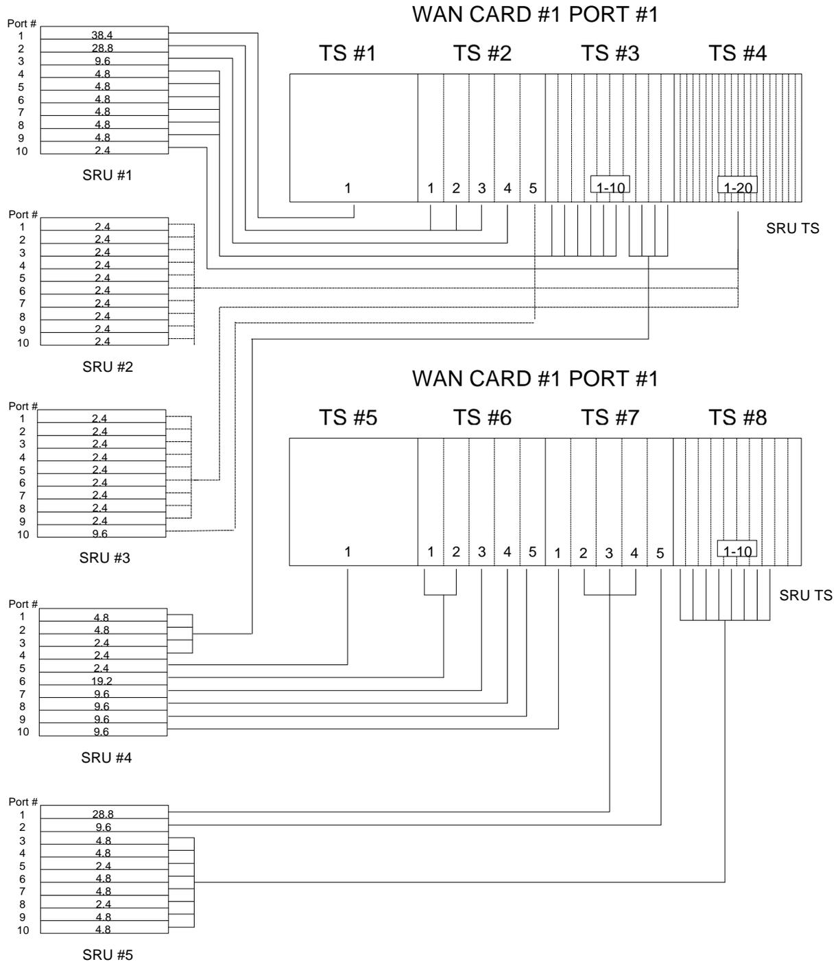
Figure SRU-7. SRU-WAN Timeslot Assignments
