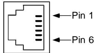
**Figure Pinouts-17. RJ11 Port**
