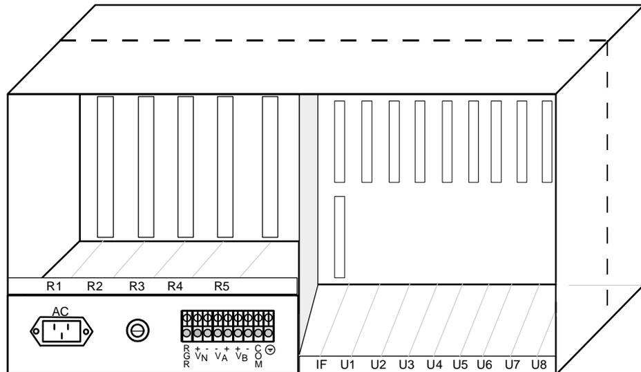
**Figure Pinouts-2. 891822/891823 Two-Sided Chassis, Back View**
