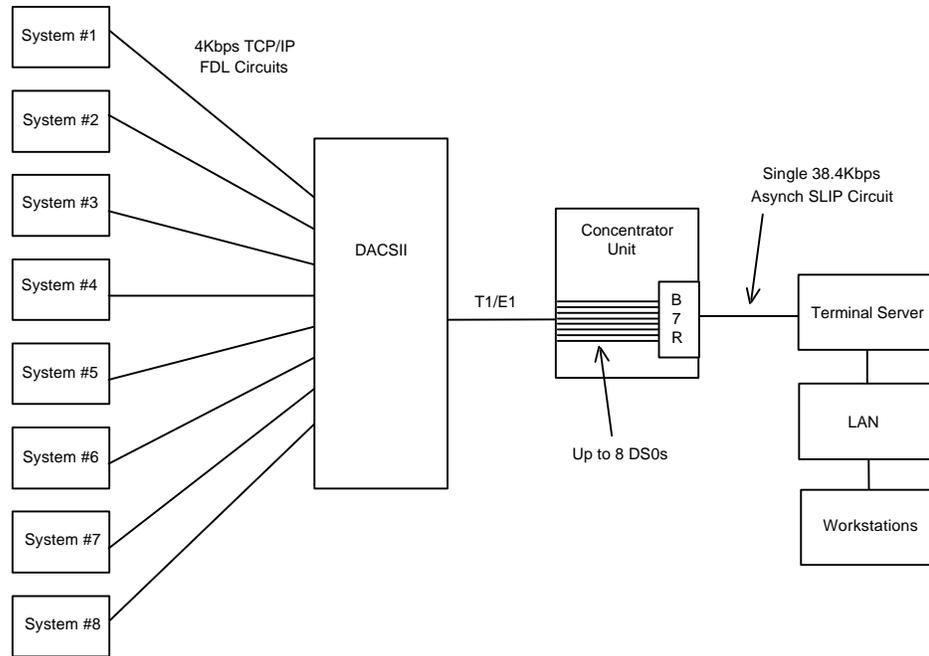
**Figure CPU-4. Typical TCP/IP Network Management System**
