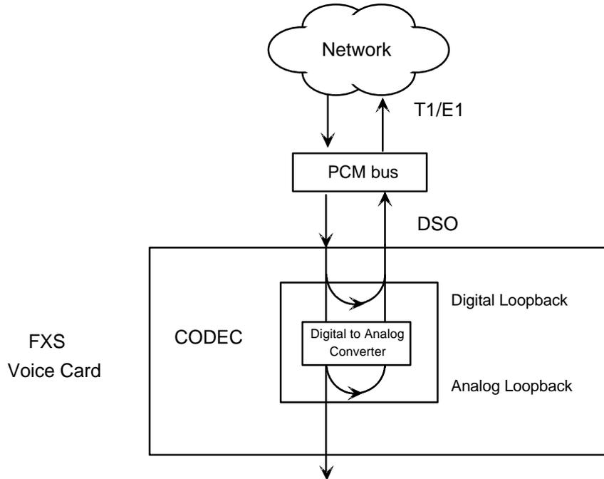
Figure FXS-2. FXS Card Loopbacks
