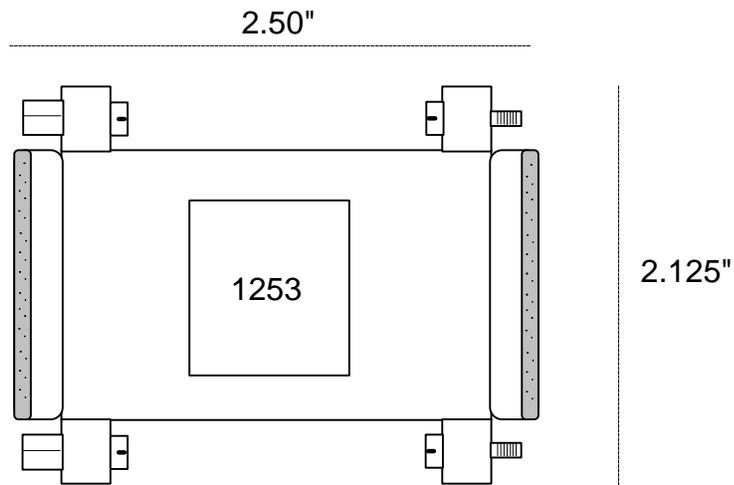
Figure HSU-14. RS530-A to RS232-E Personality Module
