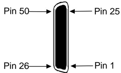
**Figure Pinouts-22. 8124 and 8125 FXS Card Connector**
