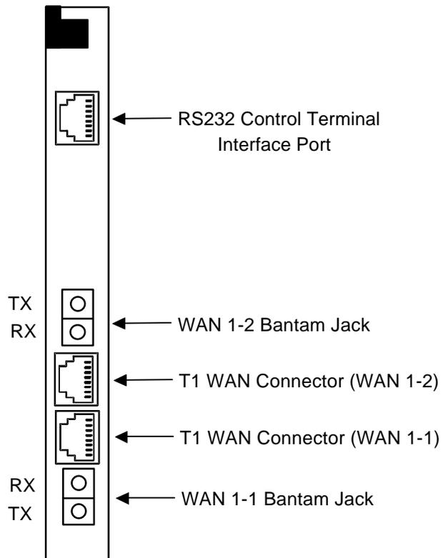
Figure Pinouts-10. 8925 Interface Card Ports
