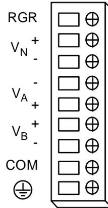
Figure Install-15. 891920 Terminal Power Connector
