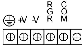
**Figure Install-9. Chassis External Power Connector (rev. C1+)**
