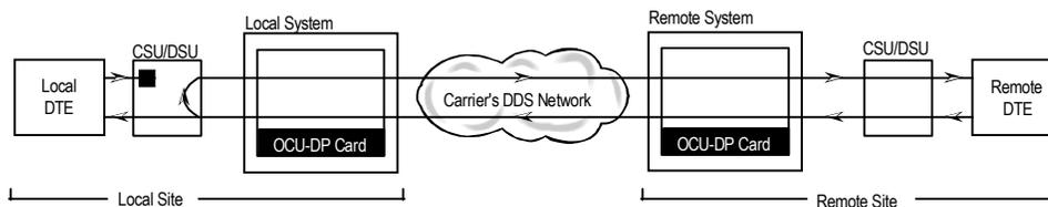
**Figure 3-11. OCU Remote Loopback (csu-u option)**
