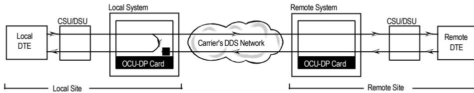
**Figure 3-6. OCU Local Loopback (dte option)**
