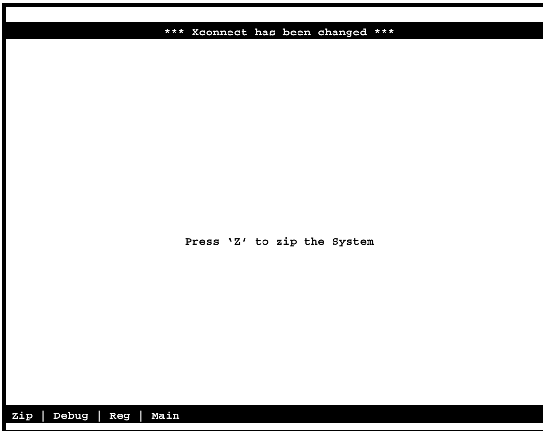
Figure 4-10. Cold-Start NVRAM Test Screen.
