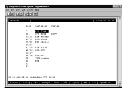
Figure 4-70. Manually Switching to a Redundant CPU
