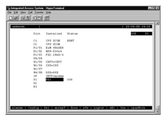
Figure 4-69. Typical Redundant-Power Supply System Main Screen
