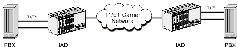
Figure 4-6. IAD using ADPCM for PBX to PBX Application
